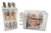
Fig 6.1.12: An electromagnetic switch
