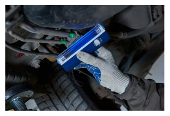
Fig 4.10.16: Leak detection using ultra-violet lamp
