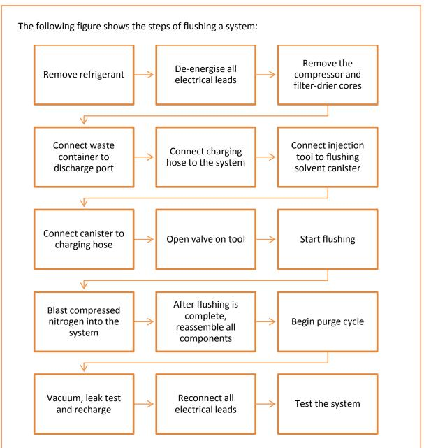
Fig 4.10.12: Steps for flushing system
