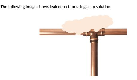
Fig 4.10.15: Leak detection using soap solution
